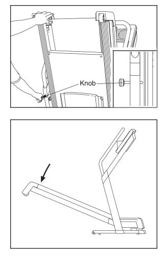
2. Hold the treadmill firmly with both hands, and lower the treadmill to the floor. To decrease the possibility of injury, bend your legs and keep your back straight.
